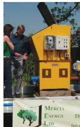
Mercia Energy biomass boiler demonstration unit
